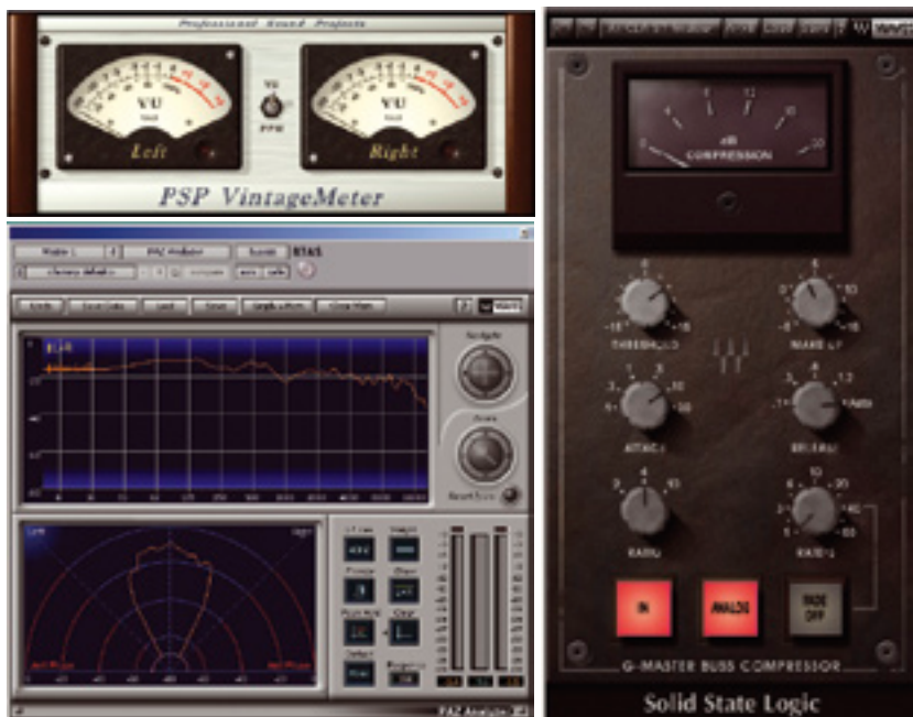
Level meters and a basic spectrum analyser plug-in can work wonders for gauging tonal imbalance in a mix.
