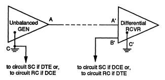
change circuits, one in each direction of transmission. Circuit SC (Send Common) is the common return for all Category II circuits having generators in the DTE. Circuit RC (Receive Common) is the common return for all Category II circuits having generators in the DCE. The waveshaping requirement to enable transmission over at least 200 feet of cable also applies here.
