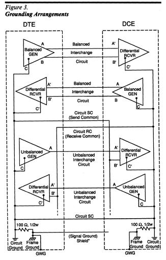
GWG is ground for the power system. \* Normally no connection to shield in DCE. Electronic Industries Association (EIA) RS-449 Interface Standard
