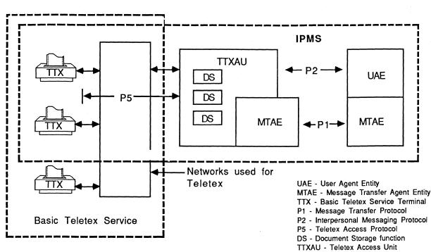
The Teletex Access Unit (TTXAU) expands the functionality of the MTAE to support terminals of an existing TTX network. Special Document Storage entities spool messages between the TTX terminals and a conventional UAE.
