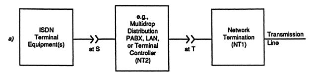
An implementation (see Figure 3a) where ISDN physical interfaces occur at reference points S and T.
