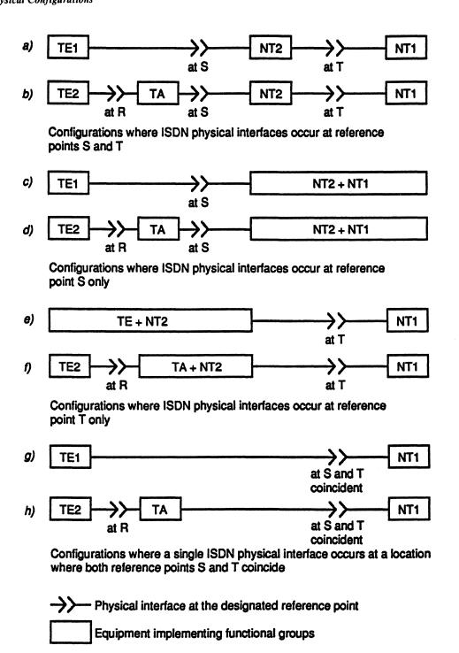
Examples of physical interface configurations at the R, S, and T reference points.
