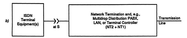
An implementation (see Figure 3c) where ISDN physical interfaces occur at reference point S but not T.
