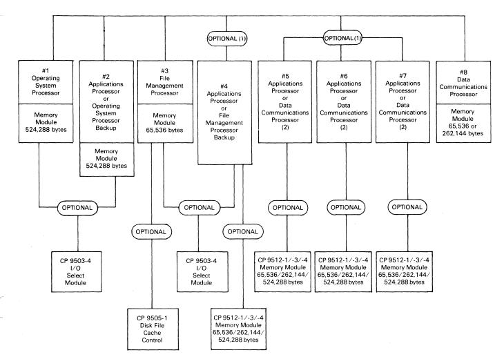
Figure 1. Schematic of CP9582/5 processor and memory options
