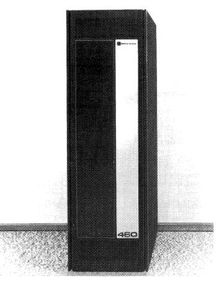
Behind the front door of the TL460 cabinet pictured above are racks of printed circuit boards that provide interfacing for up to 3121/O channels. Multiple cabinets can be cabled together chain-style, permitting one TL460 to service a maximum of 4000 channels and maintain up to 2000 cross-connects.
