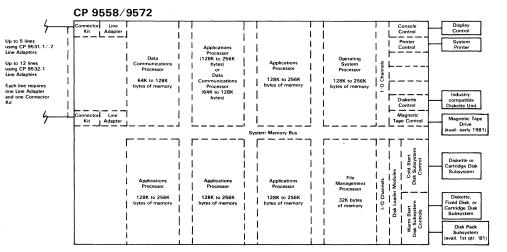
CP 9558 configuration includes one operating system processor, one file management processor, one data communications processor, and one applications processor as standard components. Two additional applications processors, or one applications processor and one data communications processor, may optionally be added, for a total system maximum of six processors, or 1.2MB of aggregate main memory.
