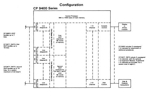
Installation of an I/O Expansion Module restricts the number of lines that can be handled by the second DCP to 4.
