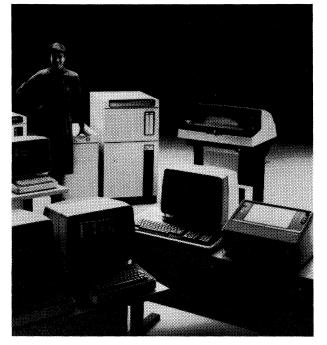
Burrough's latest CP 9500 Series offerings, Models CP 9558 and CP 9572, contain from four to eight independently operating processors that permit the system to be used in a wide variety of transaction-oriented environments. The processor system shown above includes a new Burroughs B 9494 disk drive, B 9246 line printer, and a cluster of Burroughs BMT display terminals.
