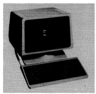
The Visual 383 provides emulation of the Burroughs TD 830 poll/select terminal. Like all of the models in Visual's display terminal product line, the 383 contains a tilt/swivel monitor and detachable keyboard.
