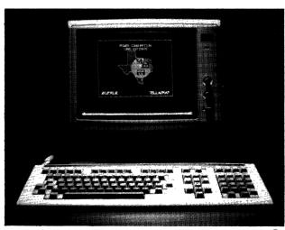
The Visual 241 is a color graphics terminal that emulates the Digital VT241. The Visual 241 supports Tektronix 4010/4014 and Digital ReGIS graphics protocols, making the unit compatible with a wide variety of graphics software packages. A 13-inch display screen with an 80/132-column display format is standard.
