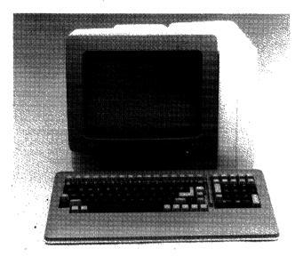
The Model 970 is TeleVideo's newest display terminal. The 970 features a special ergonomic design in which the logic boards and power supply are mounted vertically on the side of the CRT, providing true convection cooling. The screen is also balanced so that it can be tilted with the touch of a finger. The 970 is a DEC VT100 compatible terminal and features 80/132-column display capability.
