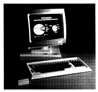
The QVT 511GX is a raster-scan color graphics terminal. It can display text or graphics in up to eight colors, selectable from a palette of 64.
