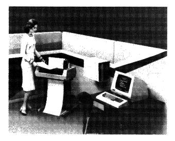
This basic Model 296 configuration consists of the controller (mounted on the wall panel), a 1920-character display, a 78-key typewriter-style keyboard with a 12-key Program Function Key cluster, and a Sprinter impact matrix printer.
