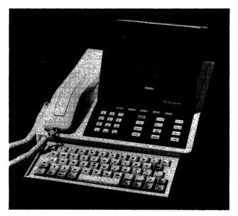
The Northern Telecom Displayphone PLUS is the newest addition to the company's Displayphone line of IVDTs. The Displayphone PLUS includes a 7-inch amber display screen, integral telephone handset, retractable keyboard, and an integral 300/1200 bps modem. The unit also includes downloadable terminal emulations of several popular ASCII terminal models.
