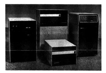
Northern Telecom provides a total of four control units for use with the 290 Display System. Remote units are: the 296C, which provides support for eight devices; the 294-51C, which supports up to 12 devices; and the 294C, which supports up to 32 devices. The local channel unit, the 294-1B, provides support for up to 32 devices.
