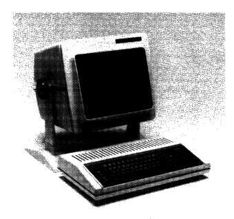
The Memorex 1377 Display Station, an IBM 3277-2 plugcompatible replacement, is highly rated by its users. Two notable features they point to are the reverse-video cursor and the tiltable display module for screen readability.
