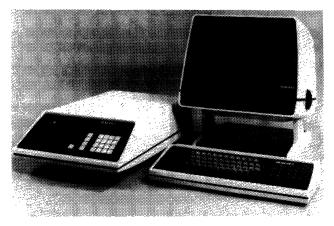
Shown with the Memorex 2076 Remote Cluster Controller, the 2078 Display Station provides a direct functional replacement for the IBM 3278 Models 1 and 2.
