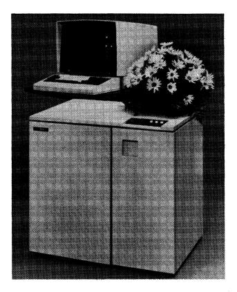
The MDS Trivex Plus 80 System includes the 8074 Remote Controller and the 8078 Display Station. Up to 32 devices can be connected to the 8074, including 8078 displays and MDS Trivex 8087 serial printers (not shown). The Plus 80 components are fully plug-compatible with the IBM 3274 controller and the IBM 3278 display, and feature SNA/SDLC protocol compatibility.
