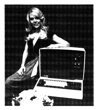
MDS Trivex's latest offering, the Model 8078 Display Station, provides plug-for-plug compatibility with IBM's 3278 display. Available in four models, the 8078 supports screen capacities of 480, 960, 1920, 2560, or 3440 characters.
