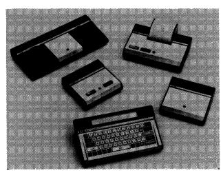
Optional peripherals provided by IXO for use with the IXO Telecomputing System include (clockwise, from upper left): the IXO Acoustic Interface; IXO 20-column Printer; IXO RS-232-C Interface; and IXO Video Interface.
