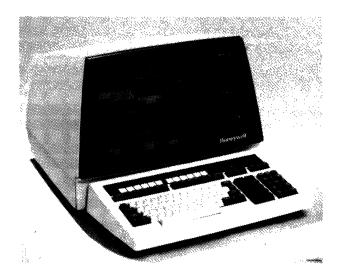
The cabinet design pictured above is the same for both the VIP 7802 and VIP 7805, which feature the 15'' diagonal display screen. The cabinet design for the 12'' screen models, the VIP 7801 and VIP 7804, is slightly different. All four models feature the 108-key typewriter-style keyboard shown here. The keyboard is detachable.
