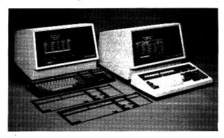
The VIP7826 (left) and VIP7816 are multiple mode terminals that feature both asynchronous and synchronous data transmission. The VIP7826 includes a multifunction, low-profile keyboard with overlays; the VIP7816 includes a standard typewriter-style keyboard.
