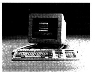
The HDS 7 is the first in a planned series of display terminals to replace the Honeywell VIP7800 Display Terminals. This multiple mode terminal features both asynchronous and synchronous data transmission, and includes a multifunction, low-profile keyboard with overlays.
