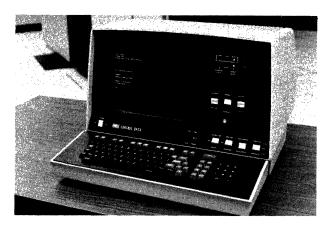
Control Data's Model 751 represents the top of its interactive terminal line. The 751 is controlled by an Intel 8080 microprocessor, is loaded with features, and can be used in a point-to-point or multipoint operation.
