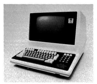
The Control Data 722 Display Terminal is a microprocessorcontrolled, asynchronous terminal for both local and remote data processing. It is intended to be the first member of a new family of operator-oriented terminals from CDC.
