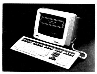
The CIT-220+ is an ergonomically designed video terminal fully compatible with Digital's VT220, VT100 and VT52. The five programmable video attributes, multimode bidirectional auxiliary port and eleven setup menus enhance this units functional capabilities. The 12-inch diagonal, nonglare screen provides 24-line by 132/80-character column display.
