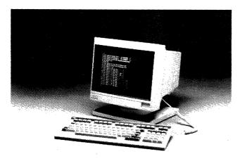
The ANT provides features normally found on other basic ASCII terminals. The unit contains a 14-inch nonglare amber screen with 24-line by 80 format and 25th status message line. It is fully compatible with the ADDS Viewpoint A2, ITT Qume QVT 101, TeleVideo 910, and Lear Siegler ADM 3A/5. The difference is the price-\$299. The ANT is currently the lowest priced alphanumeric terminal on the market.
