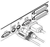
3. Locate the power cord that came with your AutoView unit. Plug it into the IEC power connector on the AutoView. Make sure that the AutoView power switch is off, then plug the other end of the power cord into an appropriate AC wall socket. This socket must be near the equipment and easily accessible to allow for unplugging prior to any servicing of the unit.
