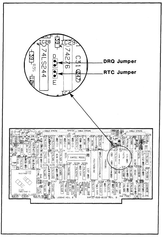
Figure 3-1: DRQ AND RTC JUMPER LOCATIONS
