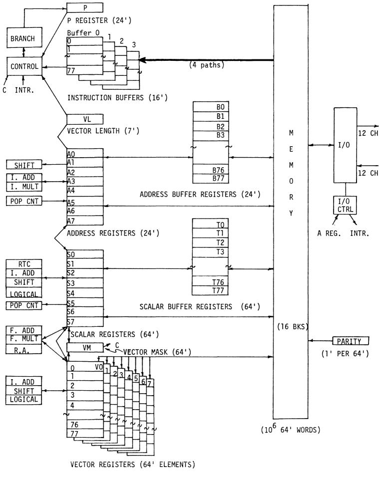
Figure 1. Registers block diagram
