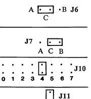
**J6** should be connected from A-C for all CompuPro drives.
