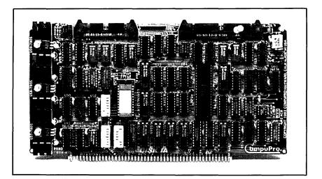
HIGH PERFORMANCE FLOPPY DISK CONTROLLER FOR 8" AND 5.25" DRIVES DISK 1A TECHNICAL MANUAL Copyright 1984 CompuPro Hayward, CA 94545
