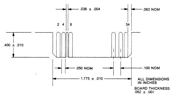
FIGURE 5. J1 CONNECTOR DIMENSIONS
