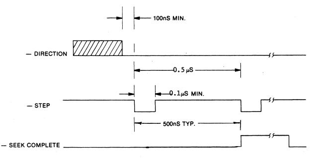
FIGURE 9. STEP PULSE TIMING
