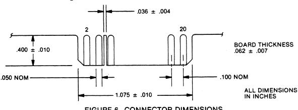
FIGURE 6. CONNECTOR DIMENSIONS
