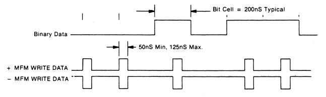
FIGURE 12. MFM WRITE DATA TIMING.
