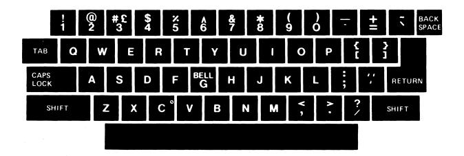
Figure 2-2. CIT-414a Standard Keyboard Keys
