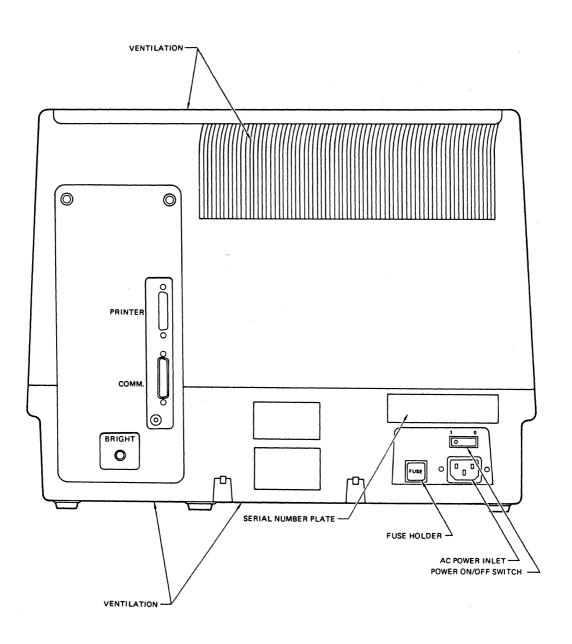
FIGURE 1-1. CIT-414a CONNECTORS AND CONTROLS
