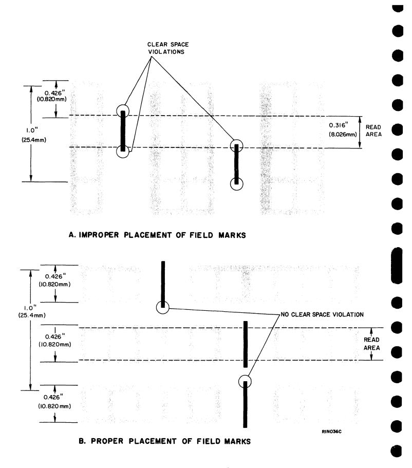
Figure 3-10. Placement of Field Marks
