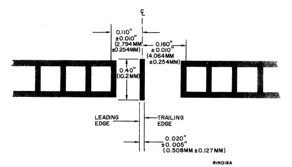
Figure 3-8. Field Mark Dimensions {for Vertical Line Spacing Densities of Two Lines per Inch or Less}
