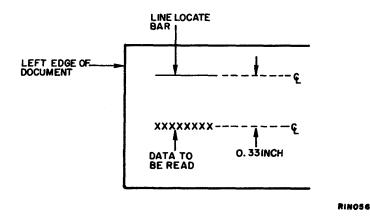
Figure 5-11. Minimum Vertical Separation Between Line Locate Bar and Data Line
