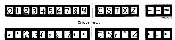
The figure four is printed with an open top.
