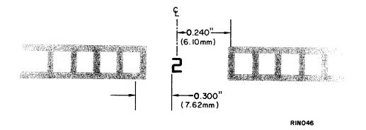
Figure 3-12. Positioning of Reference Character Serving as Field Separator
