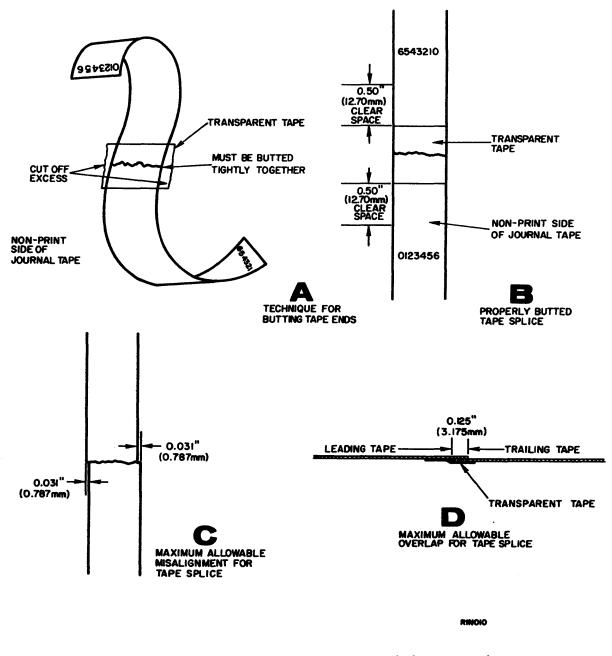
Figure 6-2. Correct Journal Tape Splicing Technique
