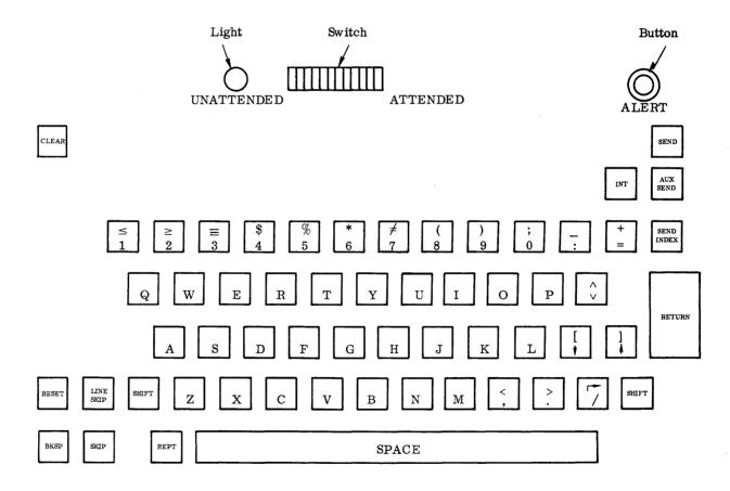
Figure 2-4. Display Standard Keyboard
