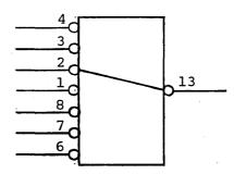
Each baud rate requires a strap from pin 13 to one of the first eight pins, depending on the rate.
