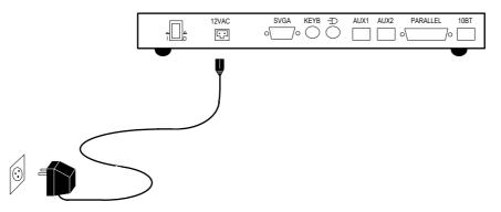
Warning: Only use the Axel external transformer supplied with your AX3000 Model 75E. Use of any other transformer may cause permanent damage to the AX3000.
