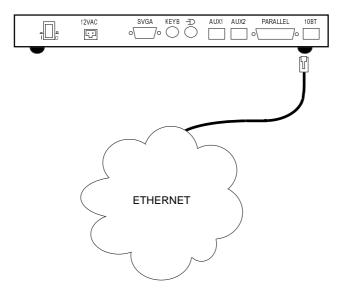
ETHERNET CONNECTION INDICATOR LIGHT: This indicator is a green LED, located next to the RJ45 connector on the rear of the terminal. It lights to indicate a satisfactory connection to the Ethernet circuit (server or hub).
