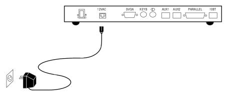
Warning: Only use the Axel external transformer supplied with your AX3000 Model 65E. Use of any other transformer may cause permanent damage to the AX3000.
