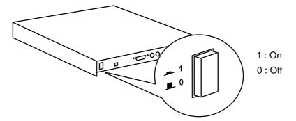
The green LED on the front of the terminal should light, and a single audible beep should be heard, to indicate that the AX3000 terminal is powered up and operating correctly.
