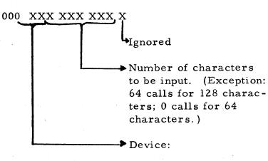
000 Flexowriter keyboard 001 Flexowriter reader 010 FACITAPE reader
