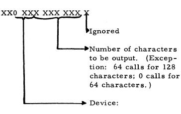
000 Flexowriter keyboard 001 Flexowriter punch 010 FACITAPE punch
