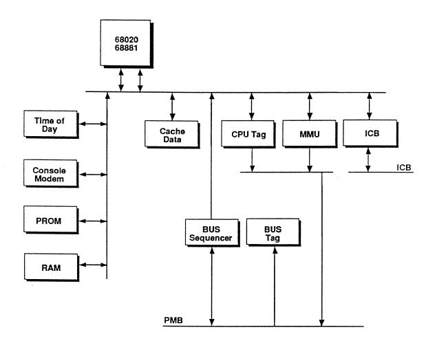
Figure 1-1. CPU32/25 Block Diagram
