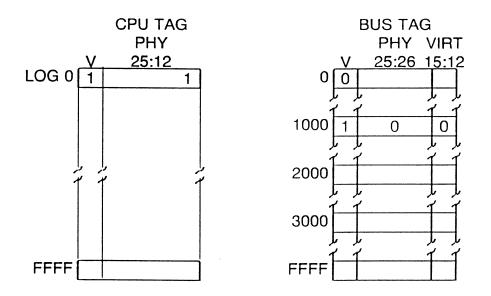
Figure 3-6. Cache Fill: Read Virtual 0 And Physical 1000
