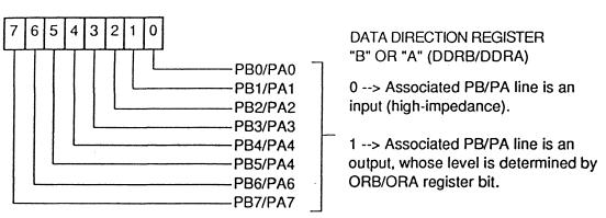
Figure 4 - Data Direction Registers (DDRA, DDRB)
