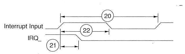
NOTE: Interrupt Input refers to either CA1, CA2, CB1, or CB2. Although timing spec #20 is shown with the rising edge of the Interrupt Input, it should be understood that this timing spec also applies when the falling edge is the active edge. Also note that timing spec #21 assumes that interrupts have been enabled for the particular Interrupt Input in question, otherwise IRQ\_ would not go active. Timing spec #22 specifies the minimum pulse width for active high and active low pulses.
