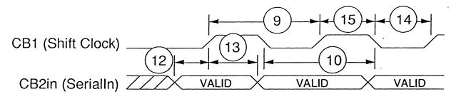
Note that when the Shift Register is programmed to shift in, the rising edge of CB1 is the active edge.
