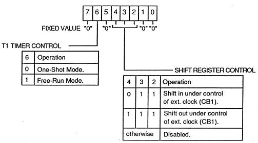
Note that bits 7, 5, 1, and 0 of the ACR are hardwired to "0". These bits are used in the 6523 VIA to select modes which are not supported in the VIA Cell.
