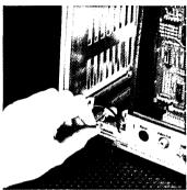
9. Hold the expansion card by the metal edge, with the green plastic facing right and the white cover facing left. Insert the bottom of the green card into the connector slot and the top of the green card into the plastic slot above the connector. Slide the card evenly into the cage as far as it will go.
