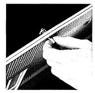
b. Insert the four tabs along the lower edge of the back panel into the slots at the base of the cabinet.
