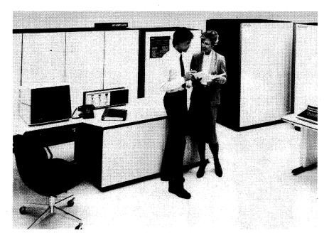
The highest performing member of the 470 line is the 470V/8 System. Shown here, this system has a cycle time of 26 nanoseconds with a performance rate estimated at between 6.5 to 7.0 MIPS (million instructions per second). All 470 systems can execute any IBM System/370 software as well as utilize System/370-compatible peripheral devices.
