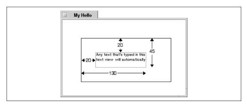
Figure 8-7. A BTextView object consists of two rectangles
