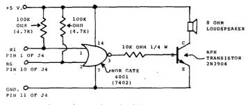
NOTE: Resistor values for 7402 IC are shown in parenthesis.
