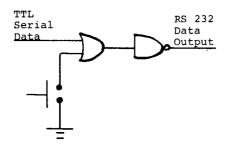
The Micro-Term terminal uses a similar setup to transmit a BREAK.
