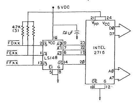
FIGURE 4: ALTERNATE DECODING FOR 2716 EPROM
