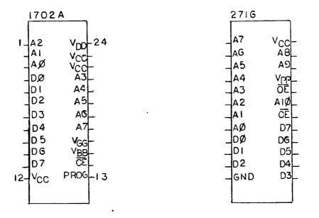
just before the second location. A jumper from the first to the third point effectively carries 02\*VMA around the PROM page decoding section. The circuit may work if pins 11 and 12 are left to float high. I chose to force them high via the five volt buss, without a limiting resistor. The five volt buss starts at B25 and B26 and by following, on top, there is another through hole in front of B38 where a logic high can
