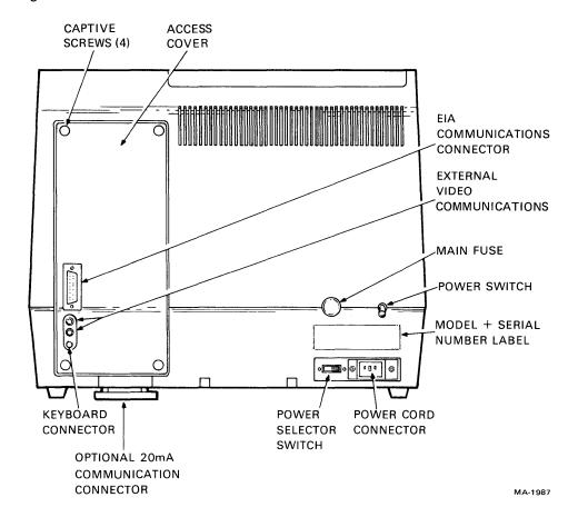
Figure 1-3 VT100 Terminal (Rear View)
