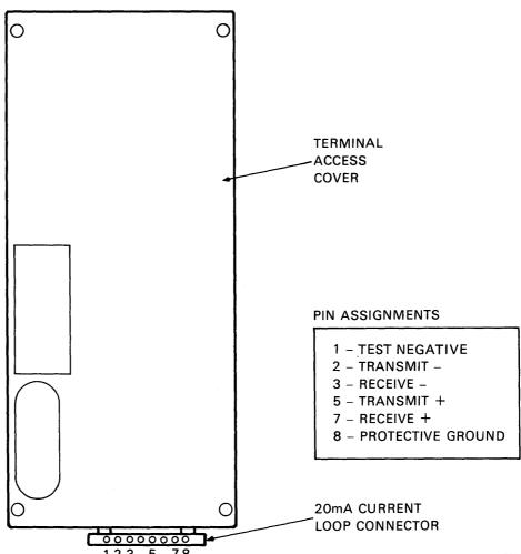
Figure 2-3 20 mA Current Loop Interface
