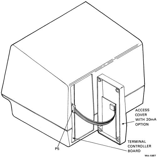
Figure 4-4 Terminal Controller Board
