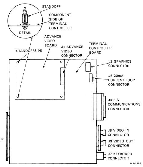
Figure 4-2 Advanced Video Option Installation
