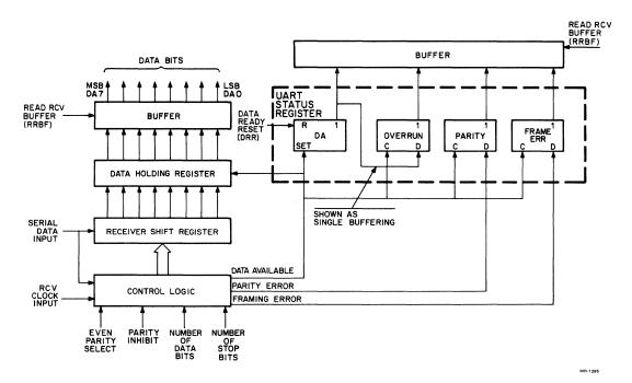
Figure 4-11 UART Receiver Block Diagram
