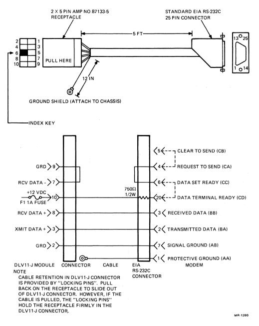
Figure 2-14 BC21B-05 Peripheral Device Cable
