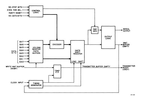
Figure 4-12 UART Transmitter Block Diagram
