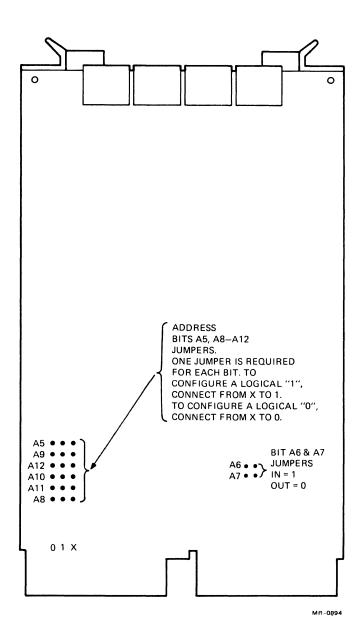
Figure 2-3 Device Register Address Jumper Locations
