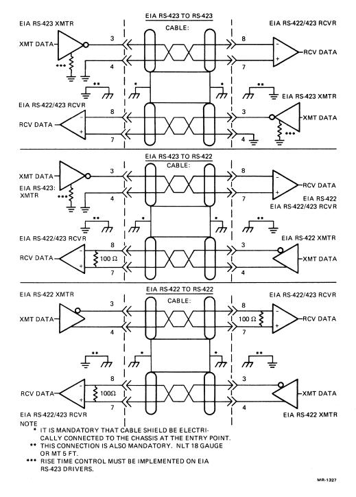
Figure 2-18 Cable Construction for DLV11-J to DLV11-J Operation
