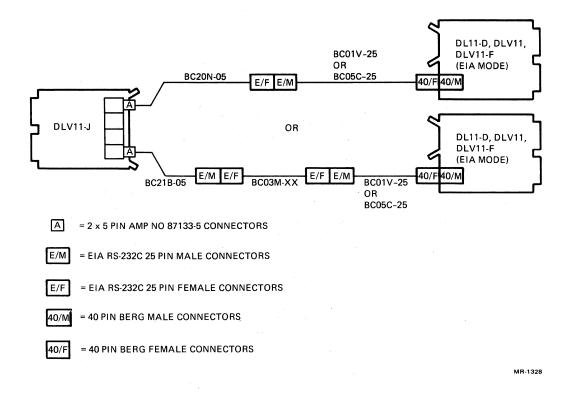
Figure 2-19 DLV11-J to SLU Module Cabling
