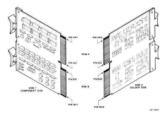
Figure 2-9 Module Contact Finger Identification
