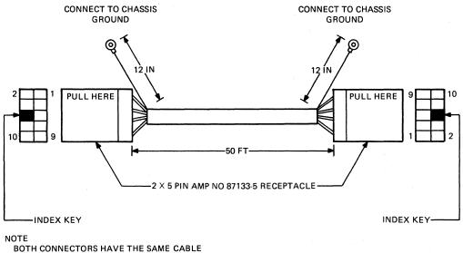
BOTH CONNECTORS HAVE THE SAME CABLE RETENTION MECHANISM. CABLE RETEN-TION IS PROVIDED BY "LOCKING PINS". PULL ON RECEPTACLE TO RELEASE.
