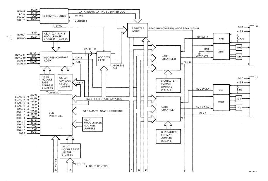
Figure 4-1 DLV11-J Block Diagram (Sheet 1 of 2)
