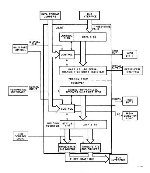
Figure 4-10 UART Signal Flow (Typical for All Channels)
