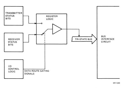
Figure 4-6 Control/Status Register During DATI
