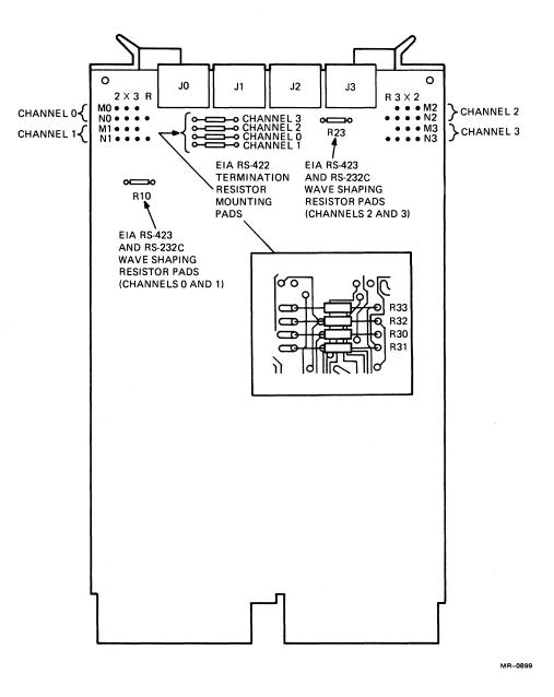
Figure 2-8 Serial Channel Signal Level Jumpers and Pads
