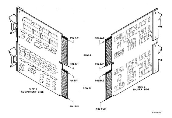
Figure 1-2 Module Contact Finger Identification
