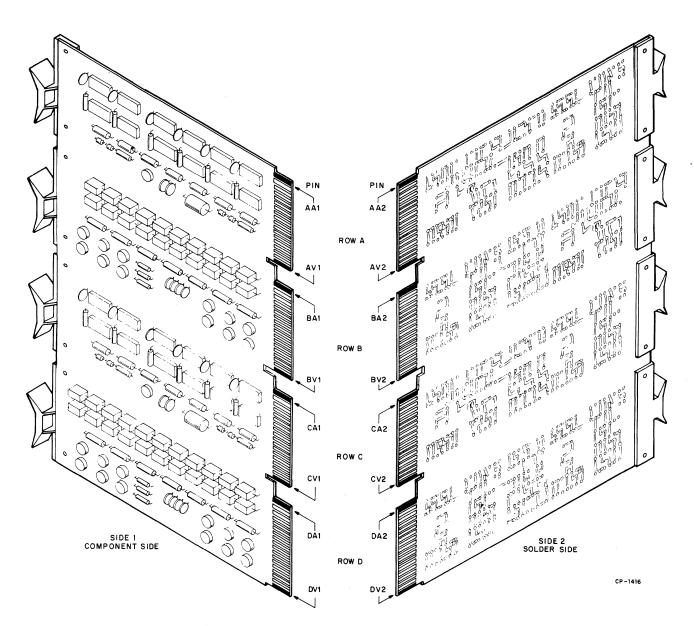
Figure 2-10 Quad Module Contact Finger Identification
