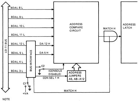
JUMPERS C1 AND C2 ARE USED TO SELECT CHANNEL 3 AS A CONSOLE DEVICE.
