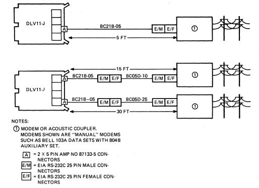
Figure 2-15 DLV11-J to Modem or Acoustic Coupler
