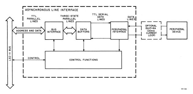
Figure 4-2 DLV11-J Data Flow, Simplified Block Diagram
