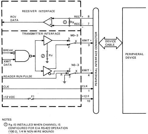
R30 - CHANNEL 0 R31 - CHANNEL 1 R32 - CHANNEL 2 R33 - CHANNEL 2 R33 - CHANNEL 3 (2) RY IS CHOSEN FOR PROPER SLEW RATE WHEN CHANNEL IS CONFIGURED FOR EIA RS-232C/RS-423 OPERATION R10 SETS SLEW RATE FOR CHANNELS 0 AND 1 R23 SETS SLEW RATE FOR CHANNELS 2 AND 3
