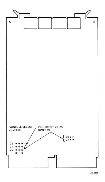
Figure 2-5 Interrupt Vector Address and Console Select Jumper Locations
