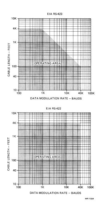
Figure 2-12 Baud Rate vs Cable Length
