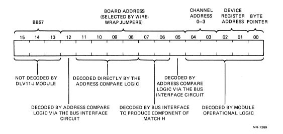
Figure 4-5 Summary of Board Address Decoding
