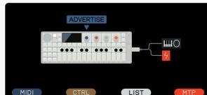
in the com screen you can access midi settings, turn OP-1 field into a midi keyboard controller, list available ble and usb midi devices. as well as access disk mode and mtp. hold shift and press the output
