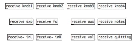
The above image shows the various paths that Organelle may use to transmit data to the current patch. These various **receive** and **receive**~ objects can be placed in your patch to fully support Organelle. A little information about each follows.
