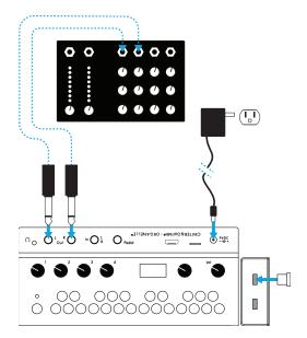
The L(eft) and R(ight) audio Out(put) ports are connected as a stereo pair to a mixer, which assumably runs to the venue's PA system, etc. (Instead of going straight to a mixer, these ports could just as appropriately be connected to direct boxes [DIs].) If there is a sound person controlling levels, you may want to leave the Volume knob all the way up, providing maximum signal for them to work with.
