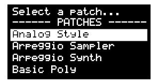
The menu screen itself comprises two sections: the system section (or system menu) at top and the patches section (or patches menu), which we see in the above image.
