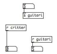
In this abbreviated example, a number 5 is received by [s guitari], and only the [r guitari] object received that 5. This is exactly how things should work.
