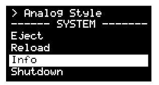
To engage one of these options, follow the same procedure as loading a patch: select the desired option by turning the Selector and then press down on the top of the Selector.
