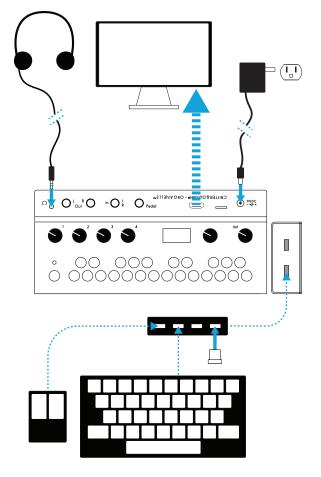
this implies the use of peripherals, such as a mouse and keyboard. This necessitates the use of a USB hub. And even without using an HDMI monitor, a USB hub would be needed if you wanted to connect multiple MIDI controllers at once, etc.
