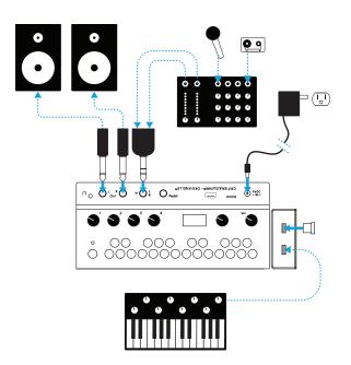
you will likely need an adapter or insert cable (aka, a Y-cable) for connecting the two devices.
